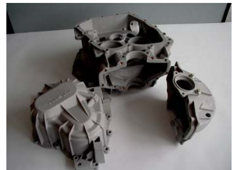
CJP gear case with threaded inserts for parts fitting and assembly inspections
