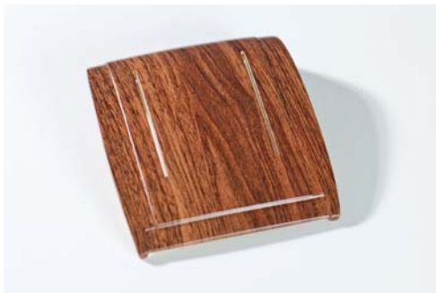
SLA model with root wood look via water transfer printing
