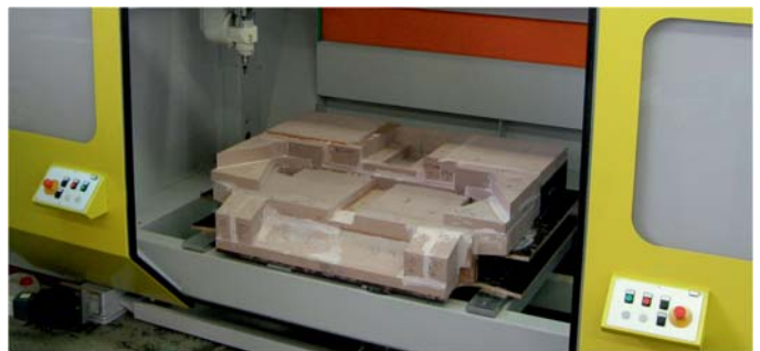
Car underbody for spray water test
