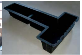
Milled mould cover made of 670 block material
